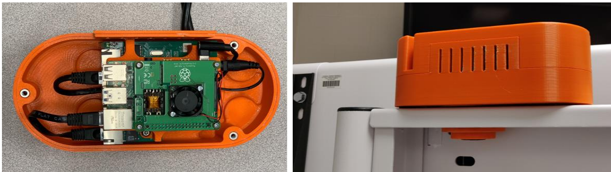
Figure 4. Enclosure Design with Modular Hardware Assembly (top view and stand mounted).
